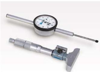
Model 1400-1 Dial Indicator (top) and Model 1400-4 Digital Depth Micrometer.
