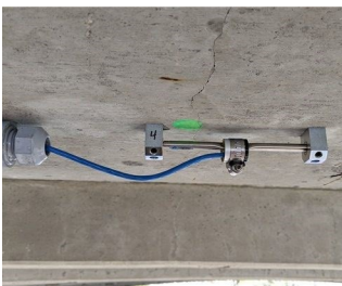
Vibrating wire strain gauge attached to the bottom flange of a girder
