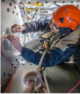
Strain gauges installation on the bridge truss.
