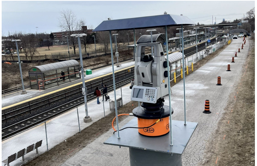
AMTS on auto-levelling tribrach
