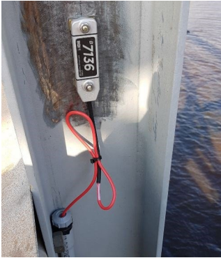
Installation of a Strain Gauge
