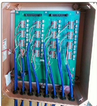
◆ Battery powered data acquisition system for vibrating wire instruments
