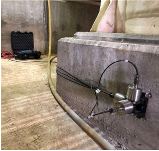
Installation SVi minimate pro accelerometer
