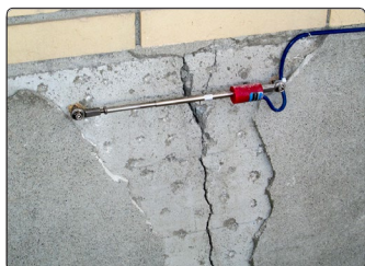
◆ Geokon 4420 crackmeter installed on basement foundation
