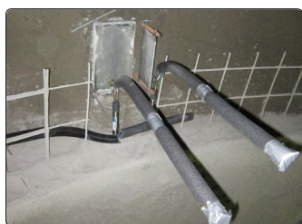
◆ Geokon 4850 NATM radial and tangential pressure cells installed at the interface of the ground and shotcrete lining
