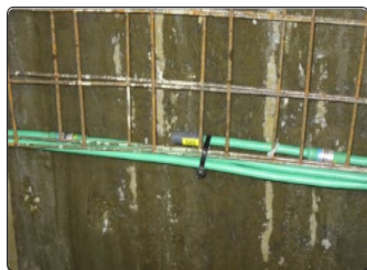
◆ Temperature measurement profile with thermistor strings installed along circumference of the frozen soil
