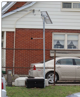
♦ Autonomous Sound and Vibration Monitor
