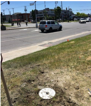
Surface monitoring instruments hidden in service boxes
