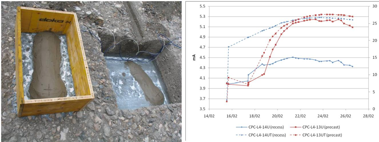
Figure 4: View and graph of precast and recessed total pressure cell installation methods test.
