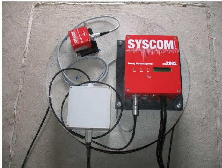
Figure 6 : Seismic tri-axial MEMS accelerometer and recorder
