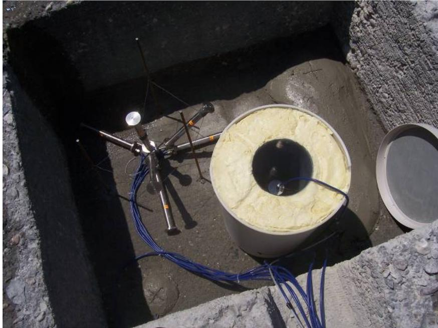
Figure 3: recess with strain gages, No stress gage
