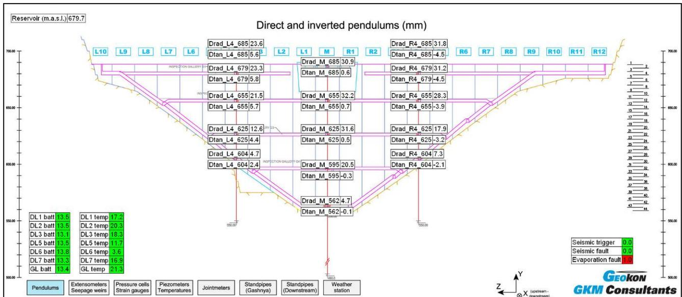
Figure 9: Virtual Mimic screen showing Pendulum measurements and location
